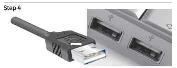
**Step 4 con't** - Connect the USB cable to any available USB port, a blue LED will illuminate when the computer is powered on.
